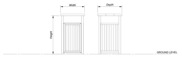
**Dimensions** Width - 580mm, depth - 580mm, height - 950mm. (sizes are approximate)
